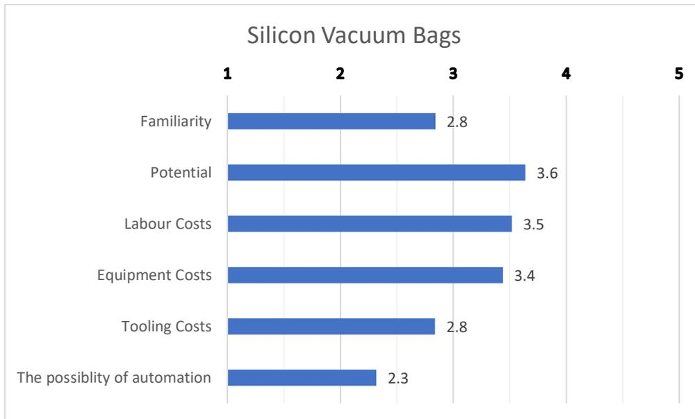
Silicone vacuum bags are mainly used in series production. With their help, we can greatly speed up the process of vacuuming the composite parts and thus reduce labor costs. Silicone bags can also be used several times and in this way we also reduce the cost of equipment in the process.
