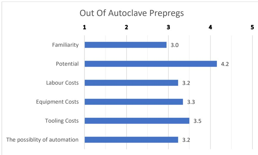
Preimpregnated fibers for use without autoclaves are fairly well known in the composite industry (59% of our respondents know and use the process). Their goal is to reduce the cost of making quality pieces by excluding autoclaves from the process, which represent a high cost on both the equipment and tooling side. Such fibers are much more ventilated in a vacuum, which means that they are adapted to the process that removes air gaps between the fibers.
