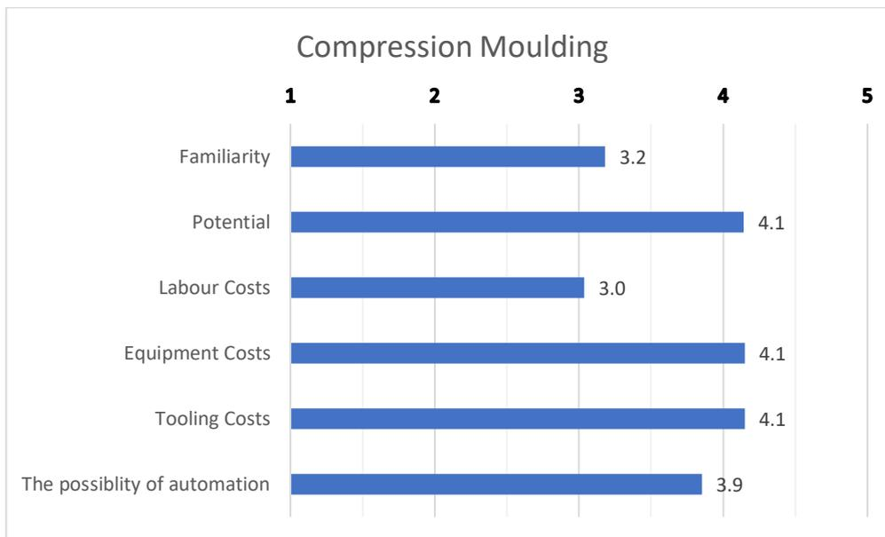
Compression Moulding is a fairly well-known process in the composite industry, 64% of our respondents know and use the process. The potential of the process is very high, because this high-volume, high-pressure production method is suitable for molding complex, fiberglass-reinforced polymer parts on a rapid cycle time. The process also allows for a high degree of automation.
