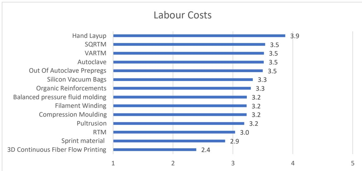
Our respondents agree that the Hand Layup is the process with the highest labor costs. This is reasonable, since with Hand Layup, all phases of the process are carried out manually, which requires a large and skilled workforce, which in turn means high labor costs. Additionally, due to manual labor, the cycles between composite parts are also long, which makes the process unfavorable for mass production.
